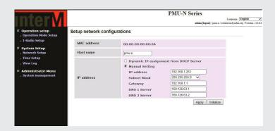
The web-browser interface will allow you to setup and configure the Network Settings, Security, Date/Time, User definable Web Stations, Timed Broadcast Automation, Firmware Update, Maintenance and Log Files. Through the web-browser interface, you can easily select the desired channel to broadcast.
